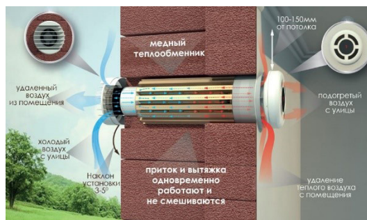
Figure 22: Individual ventilation wall mounted unit with heat recovery (sample 1)
